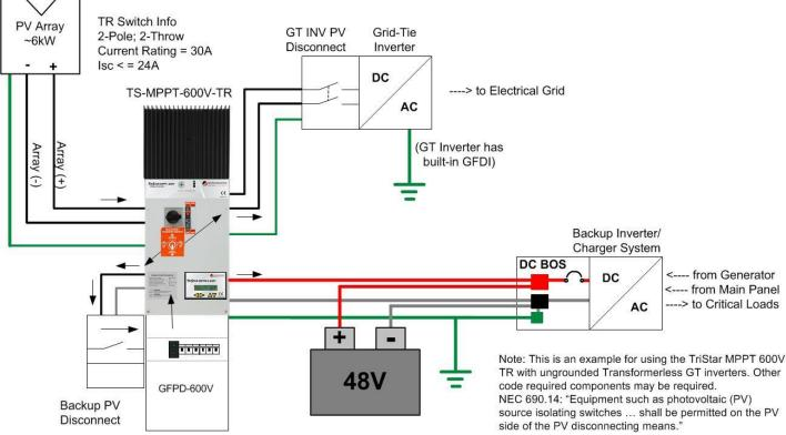
Disclaimer: These diagrams are a general overview and not intended to be a substitute for the installation and operation manual. Please read all of the instructions and cautions in the manual before beginning installation. Installation of this equipment should only be performed by qualified individuals. http://www.morningstarcorp.com/wp-content/uploads/2015/05/Operation-Manual-TS-MPPT-600V-48-DB-TR\_GFPD\_v1.1.pdf
