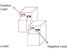
Parallel Connection, 12V 200Ah bank Increases Ah, Voltage stays the same.
